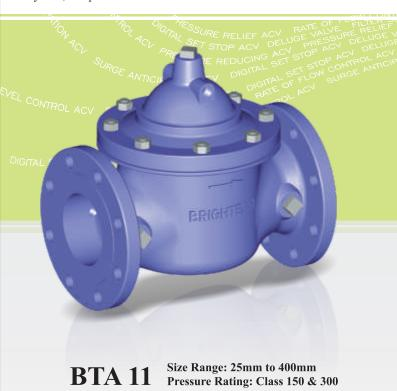
The **Automatic Control Valve**, the word is self explanatory. It is a highly engineered Automatic Control Valve knowledgeably designed to operate of the line pressure or if desired, from an independent power source. Actrol valves are hydraulically operated, diaphragm actuated for multi-function control of non corrosive, non abrasive fluids.
